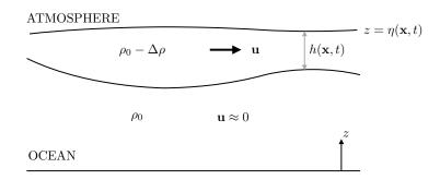
The evolution of the horizontal velocity  $\mathbf{u} = (u, v)$  and thickness h of the upper layer are determined by the *Boussinesq reduced-gravity equations*, which take the form
